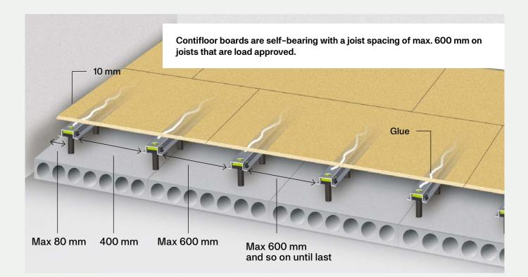
The boards are carefully glued to the joists with an MS polymer adhesive, Kiiltoflex N20, Casco Superset or similar adhesive from another supplier. V20 quality-classed Cascol 3304 adhesive is used in the chipboards' T&Gs. Cascol 3303 is used for temperatures below + 10°C. V313 quality-classed Cascol outdoor 3337 adhesive or other equivalent "class D3" adhesive is used in the T&Gs.
