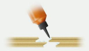
\* This gluing also applies to Tempo flooring
